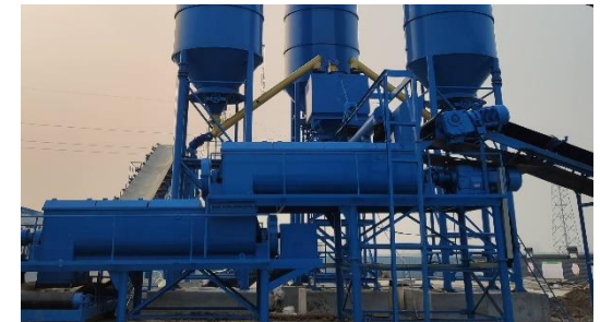
Solidified Soil Mixing Equipment
